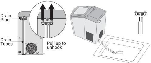
Reattach the Drain Plug to the Drain Tubes. Attach the Drain Plug back into the two slots at the back of the Ice Maker as illustrated in the "HOW TO USE" instructions earlier in this manual.
