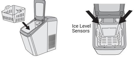
**6** Close the Front Lid. Press the "ON/OFF" key and the **\*** indicator will illuminate with a solid light, indicating that the ice-making process has begun.
